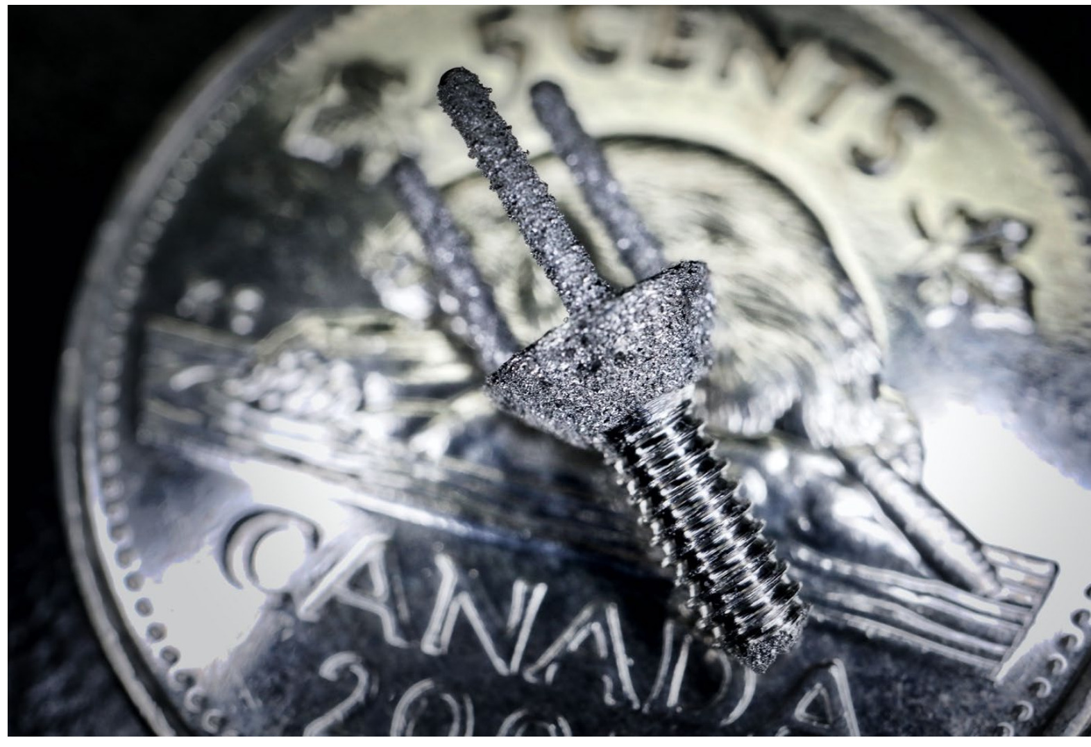
Figure 1. Novel dental implant abutment scaled against a Canadian nickel (with 20mm diameter).
